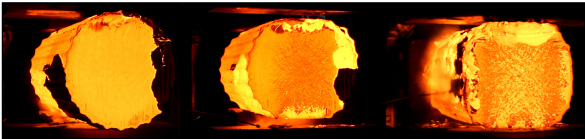
Figure 19 : Initial forming: Steps for obtaining a square base
