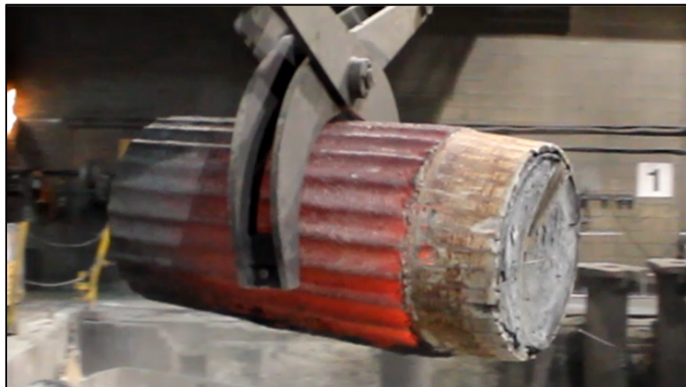
Figure 17: 63" cast ingot after demoulding
